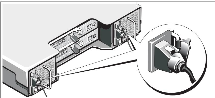
Secure the cable(s) firmly to the bracket using the provided strap.
